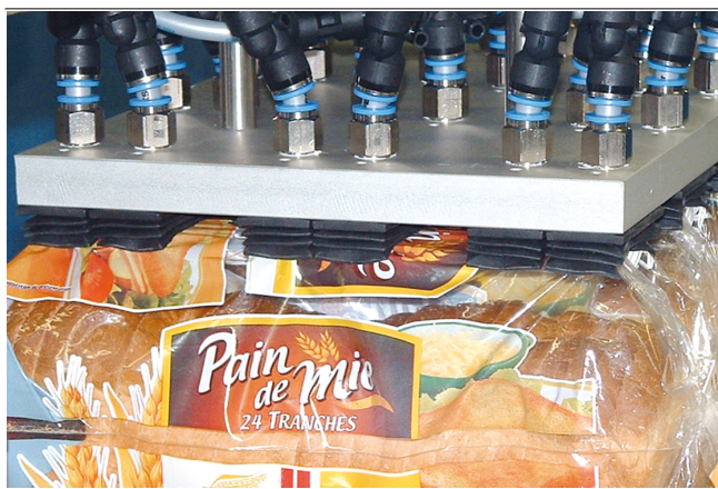
Bellows suction cups FSGB-R being used for handling of packing materials
